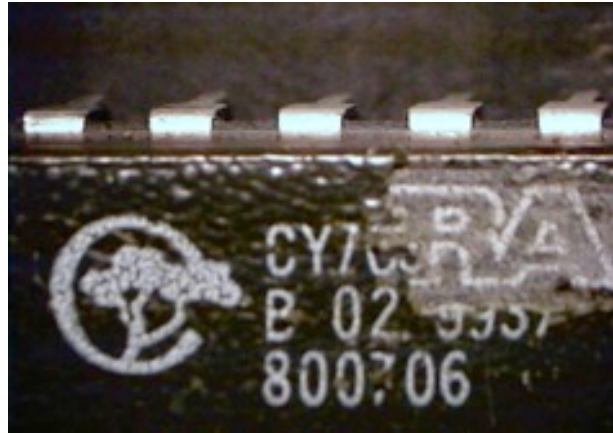
Figure 5. This chip was coated and remarked. The original logo is partially visible. (AERI, 2013)
